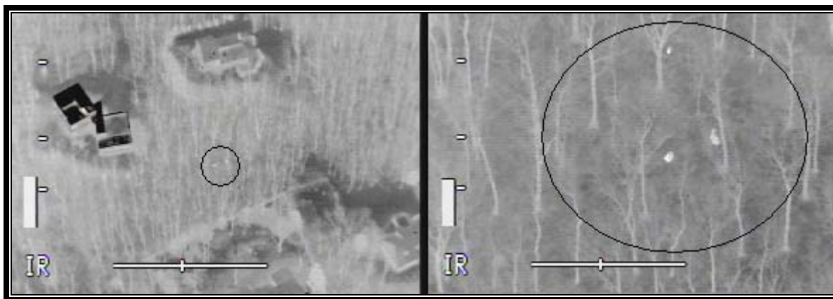
Figure 2. Three deer were bedded between homes on Shelter Island, NY in March 2007 during the infrared survey conducted by Vision Air Research, Boise, ID. The left infrared image is taken with the wide field of view while the right image is taken by switching to the narrow field of view.
