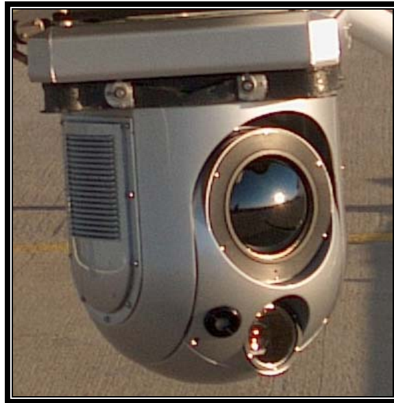
Figure 3. Polytech Kelvin 350 II gimbal with infrared sensor (upper, larger lense) and natural color video camera (lower, smaller lense) use for the aerial infrared deer survey.
